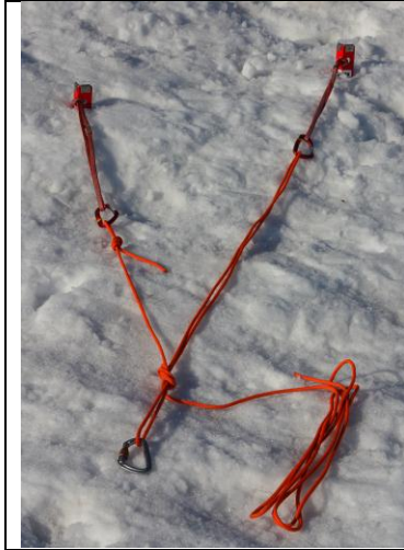
Figure 1.24: Equalizing unequal length anchor legs by doubling the cordage on the long leg.
