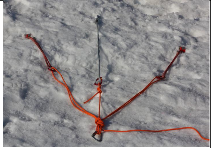
Figure 1.25: Because it is aligned with the direction of pull, the middle picket in this three point anchor receives most of the load. Doubling the cordage on the other two legs helps compensate for this. The long Spectra sling also helps.
